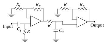
In order to get a lower cut-off frequency of  $150\,Hz$  and an upper cut-off frequency of 10kHz, the appropriate values of  $C_1$  and  $C_2$  respectively are
