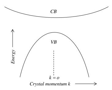
At finite temperatures the bottom of the conduction band (CB) is partially filled with electrons (e) and the top of the valence band (VB) is partially filled with holes (h). If an electric field is applied to this solid, both e and h will start moving. If the time between collisions is the same for both e and h, then
