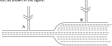
Two pressure gauges attached at the points A and B (see figure) show readings of  $P_A$  and  $P_B$ respectively. If the radius of the tube at the points A and B is 0.2 cm and 1.0 cm respectively, then the difference in pressure  $(P_B - P_A)$ , in units of dyne cm<sup>-2</sup>, is closest to
