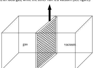
If the partition is removed and the ideal gas is allowed to expand and fill the entire container, then the entropy per molecule of the system will increase by an amount
