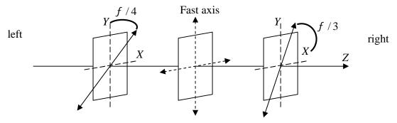
The apparatus consists of (from left to right) a polariser with transmission axis at  $\frac{f}{4}$  w.r.t. y-axis, followed by a quarter-wave plate with fast axis along the y-axis and finally, a polariser with transmission axis at  $\frac{f}{3}$  about the x-axis.
