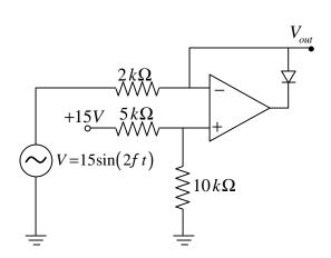
In the above circuit, which of the following is the maximum value, in Volts, of voltage at  $V_{\text{out}}$ ?
