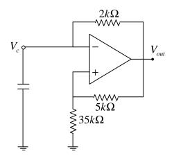
For the parameters indicated in the figure, the ratio of the maximum voltage at  $V_{out}$  to the maximum voltage at  $V_C$  is
