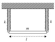
If the springs can move only in the vertical direction, the frequency of small oscillations of the rod about equilibrium is given by
