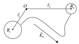
If the wire cannot support a net charge and two spheres are separated by distance much larger than the radii of each of them, the induced dipole moment in the system would be
