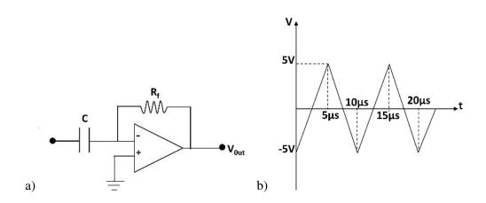
determine the output voltage waveform.
