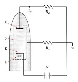
the electrons strike the plate and contribute to the plate current  $i_p$ .
