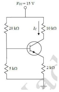
The current  $I_C$  will be \_\_\_\_\_mA. (Rounded off to two decimal places)
